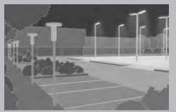
**Column luminaires and light pillars** provide technical and decorative outdoor lighting. The mounting height and the distance between the luminaires are the factors which determine the illumination of the areas and paths.
