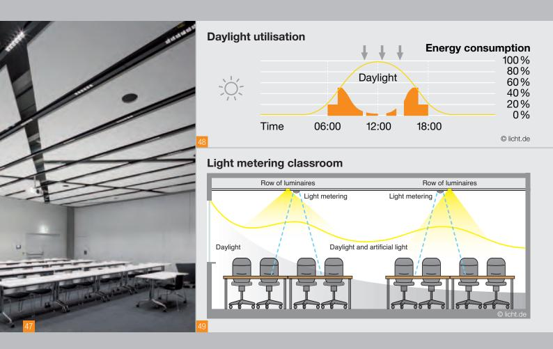
tion (see Lighting System Design Process page 68). Light management systems which work with daylight sensors only add supplementary brightness to the room with artificial light when necessary.
