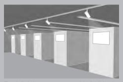
**Track lighting systems** provide flexibility in different room situations. Luminaires or spotlights can be inserted at any point on the track using an adapter, providing light to wherever it is needed.
