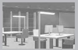
Mobile and desk lamps can be positioned as required to illuminate individual workstations and should therefore be individually dimmable. They are available with direct and indirect light distribution.
