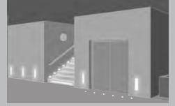
**Recessed wall and floor luminaires** are often used to highlight danger zones.
