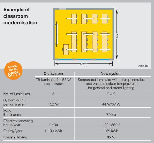
The effective operating hours are based on constant daylight-dependent control of the lighting to a target value of 500 k and on the light being switched off when sufficient daylight is available or when no-one is present.
