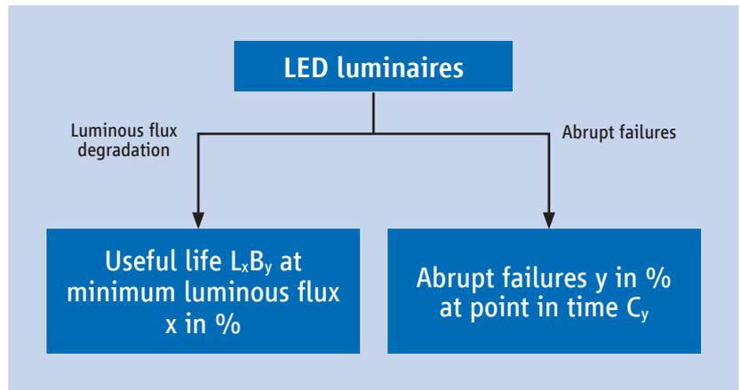
**Fig. 12b: Longevity criteria of LED luminaires for median useful life**
