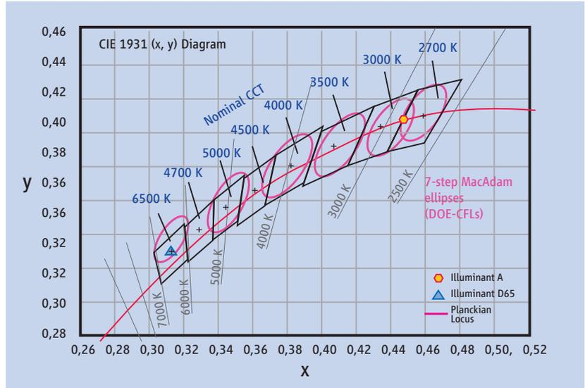
ellipse. Care should be taken to ensure small colour differences – especially for lighting applications where individual light sources are not far apart and can be seen simultaneously.
