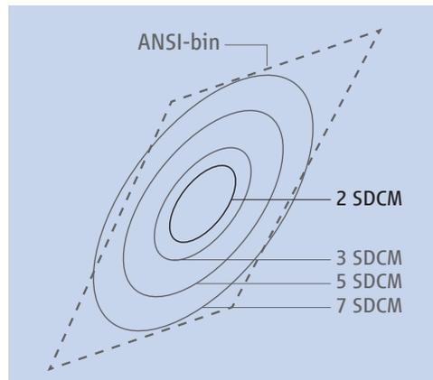
The colour coordinate tolerance of light sources is thus assessed using the steps of MacAdam ellipses (also referred to as SDCMs – Standard Deviations of Colour Matching). For compact fluorescent lamps, for example, international standards recommend a tolerance of at most a 7-step MacAdam ellipse (synonymous with 7 SDCM). From 3 SDCM upwards, differences are perceptible between colours at the edge of the ellipse and the colour at its centre.
