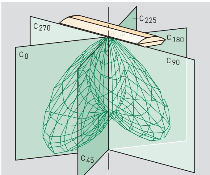
**Fig. 4: Example of the luminous intensity distribution of a streetlight**
