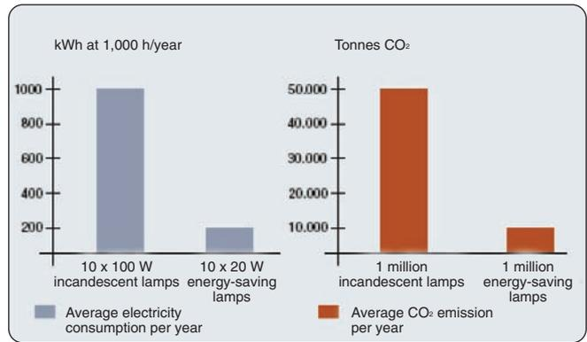
*Incandescent lamps vs. energy-saving lamps: power consumption and CO<sub>2</sub> emissions*
