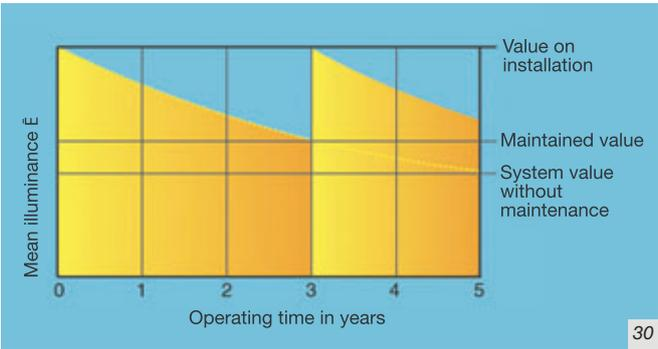
The maintained value is the local average illuminance at which the system requires maintenance. Example: maintenance interval 3 years.
