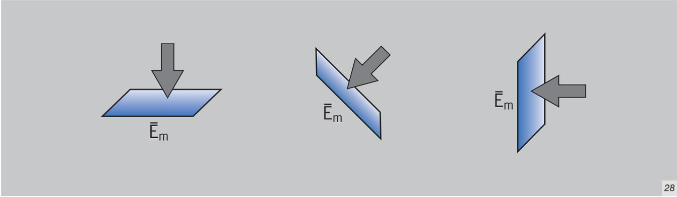
The planes on which primary visual tasks are performed may be horizontal, vertical or inclined – standard illuminance requirements  $\bar{E}_m$  apply analogously.
