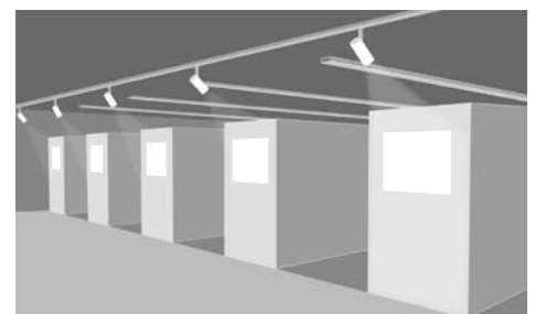
Power track systems provide flexibility for rooms where room situations change. Luminaires and spots can be mounted on adapters at any point on the track to deliver light precisely where it is needed.
