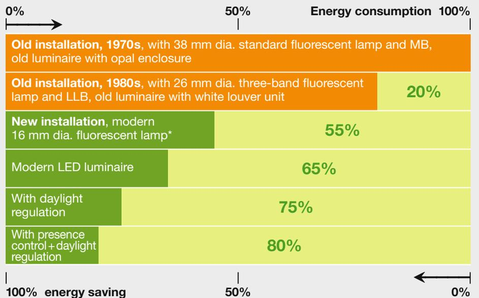
\* Fluorescent lamp operated by EB with very low power loss, energy-efficient direct or direct/indirect luminaires with modern optical control technology
