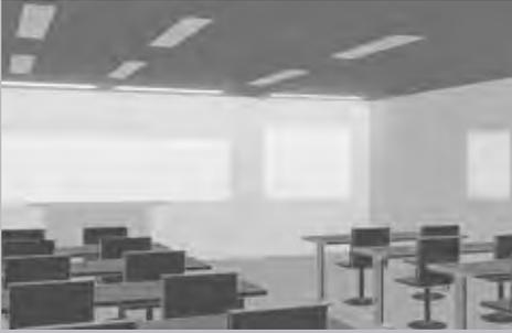
**Wallwashers** provide homogenous illumination of walls or board surfaces. They are therefore ideal for light-coloured vertical surfaces.
