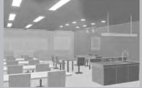
The fixtures of **recessed luminaires** are flush-mounted in the ceiling, wall or floor. Accordingly, only the light itself can be seen, with the housing of the luminaire becoming practically invisible.
