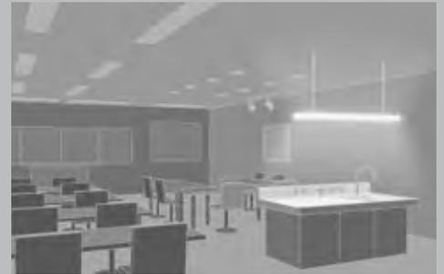
**Pendant luminaires** are mounted at a distance below the ceiling and serve as design elements in a room. They provide direct/indirect light distribution and come in a wide variety of designs.
