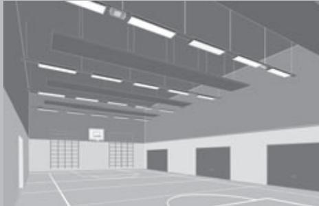
**Shock-, impact- and ball-proof luminaires:** Luminaires in sports halls must be ball-proof so that they do not break and parts do not fall off if hit. Shock- and impact-resistant lights can withstand high levels of mechanical impact.
